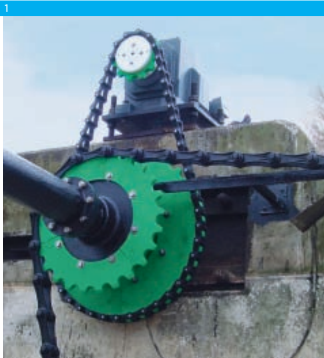
2 Drive shaft idler with maintenance-free and self-adjusting bearing
